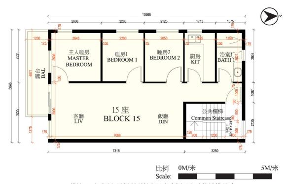
備註:平面圖之尺規所列數字以毫米標示之建築結構尺寸。 Note: The dimensions of floor plans are all structural dimensions in millimeter.
