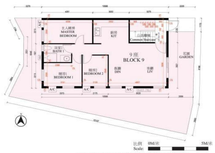
備註:平面圖之尺規所列數字以毫米標示之建築結構尺寸。 Note: The dimensions of floor plans are all structural dimensions in millimeter.
