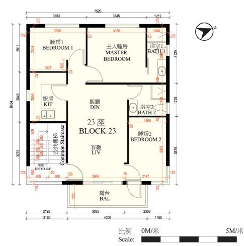
備註:平面圖之尺規所列數字以毫米標示之建築結構尺寸。 Note: The dimensions of floor plans are all structural dimensions in millimeter.
