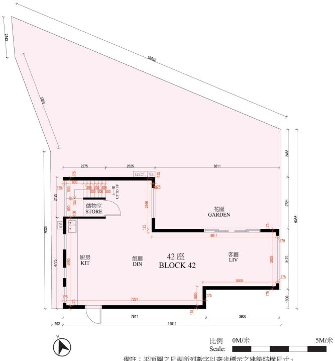
備註:平面圖之尺規所列數字以毫米標示之建築結構尺寸。 Note: The dimensions of floor plans are all structural dimensions in millimeter.
