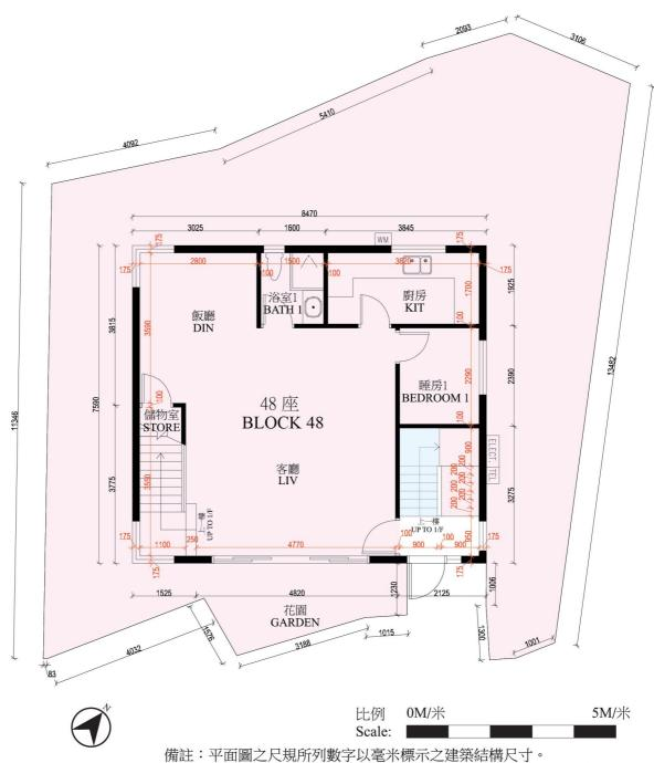
備註:平面圖之尺規所列數字以毫米標示之建築結構尺寸。 Note: The dimensions of floor plans are all structural dimensions in millimeter.
