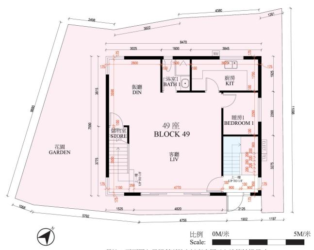
備註:平面圖之尺規所列數字以毫米標示之建築結構尺寸。 Note: The dimensions of floor plans are all structural dimensions in millimeter.
