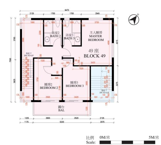
備註:平面圖之尺規所列數字以毫米標示之建築結構尺寸。 Note: The dimensions of floor plans are all structural dimensions in millimeter.
