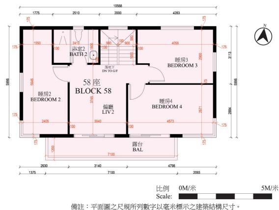
相註·十回圖之八飛的列數子以笔不標不之建架範構入了。 Note: The dimensions of floor plans are all structural dimensions in millimeter.
