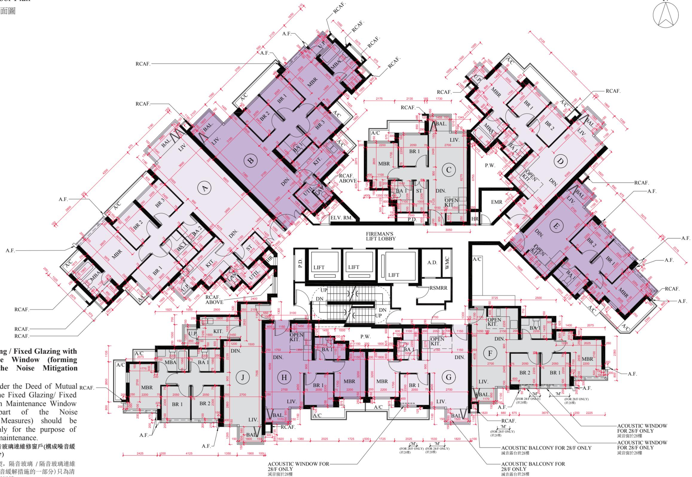
Fixed Glazing / Fixed Glazing with Maintenance Window (forming part of the Noise Mitigation Measures)
