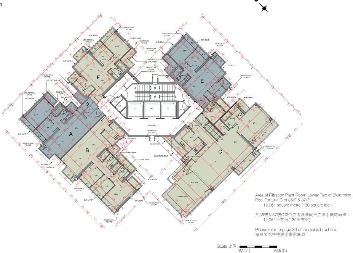
Note: The dimensions in the floor plan are all structural dimensions in millimeter. 備註:樓面平面圖之尺規所列數字為以毫米標示之建築結構尺寸。
